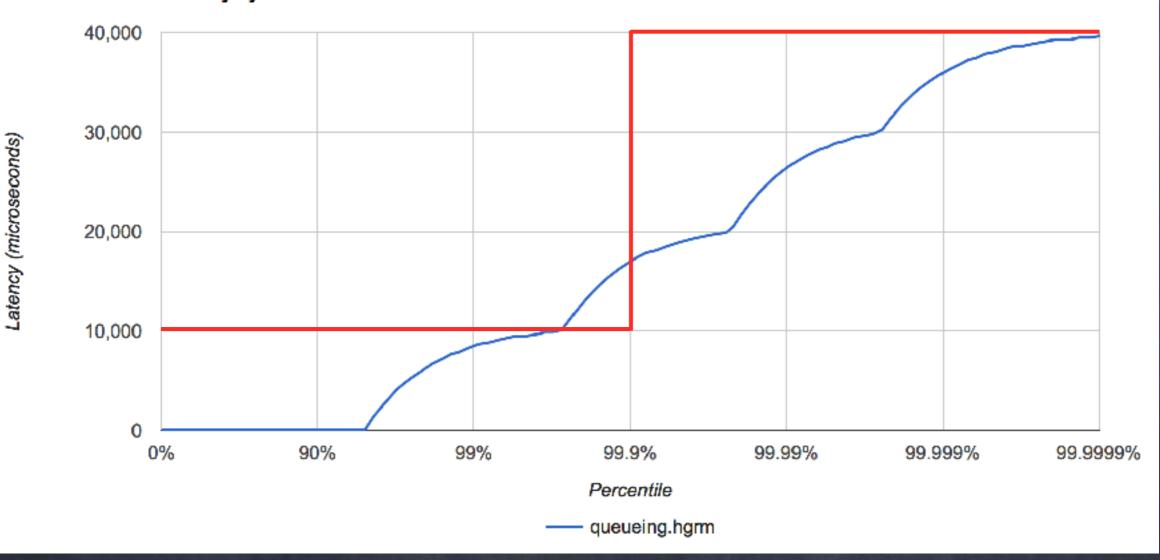
200 usec service time, 5K msg/sec capacity 250 requests/sec, arriving in bursts of 50
